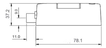
Figure 5. Dimensions of the MTX-HSDPA-EU3 terminal in mm
