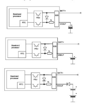
The MTX-HSDPA-EU3 can accommodate this battery or super-cap inside, and the MTX-HSDPA-EU3 can be ordered with this special option by request. Please contact <a href="mailto:gsmsupport@matrix.es">gsmsupport@matrix.es</a> about this request.
