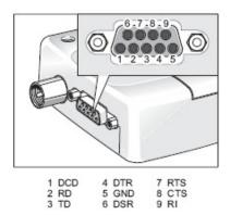
MTX-HSDPA-EU3 Terminal is designed for use as a DCE. (data circuit-terminating equipment) based on the conventions for DCE-DTE connections it communicates with the customer application (DTE- data terminating equipment) using the following signals:
