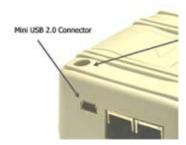
The USB I/O-pins are capable of driving the signal at min 3.0V. They are 5V I/O compliant. To properly connect the module's USB interface to the host a USB 2.0 compatible connector is required. Furthermore, the USB modem driver delivered with MTX-HSDPA-EU3 must be installed as described below.
