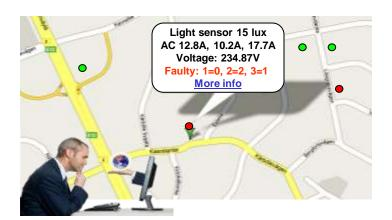
Information about lighting system problems, such as burnt lamps or faulty fuses could be forwarded to desired mobile phone or e-mail. Faults could be detected automatically to create work orders or you can make free-form orders for maintenance personnel. Browser is able both to track fault's condition and repair progress.
