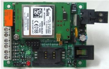
The **Pix-Cell** is a high performance, programmable Cellular Single Board Controller, that offers built-in digital and analog I/O combined with GSM/GPRS connectivity in a compact form factor. The heart of the GSM controller is a Microchip PIC18F6722 operating up to 32MHz which provides fast data processing.
