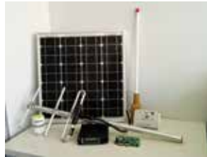
Weather station buoy with GPS and RF
