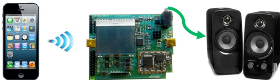
Fig.4: In addition to IoT applications, Econais' WiSmart platform offers cost-effective solutions for wireless headphones, speakers and other Wi-Fi audio products (WiSAudio). Reference hardware/software designs are also available which enable a Smartphone or PC to stream digital audio files to any stereo system within range of a home's Wi-Fi network. (Courtesy of Econais)
